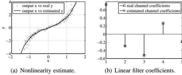
**Fig. 5.** Identification results on the  $1 \times 3$  Wiener SIMO system. (a) shows the noisy output  $x_3[n]$  vs. the real internal signal  $y_3[n]$ , and  $x_3[n]$  vs. the estimated  $\hat{y}_3[n]$ . (b) shows the estimated filter coefficients of  $\mathbf{h}_3$  vs. the real coefficients.
