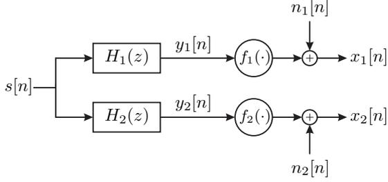
**Fig. 2.** A SIMO system consisting of 2 Wiener systems.
