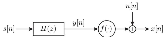
**Fig. 1.** A Wiener system with additive noise  $n[n]$ .
